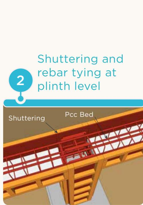
**2** Shuttering and rebar tying at plinth level
